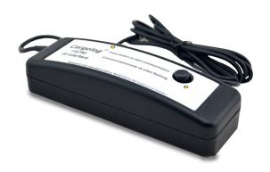
Use the IR-to-USB Interface, TopCom to connect the Cargolog® device equipped with topside IR communication to your PC. It is placed directly on top of the Cargolog® device, and you can use it even when the device is mounted in the metal case and installation bracket.
